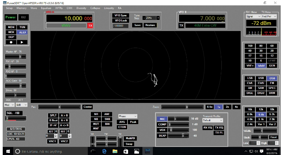
Figure 1 — You can use your SDR software phase display to adjust the receiver VFO to match the FMT signal frequency. Here, the phase display of the FlexRadio Systems PowerSDR is shown using the author's OpenHPSDR receiver. The white figure in the middle of the display shows phase error between the received signal and the receiver VFO revolving once per hertz of frequency error. Each revolution per second is an error of one hertz.
