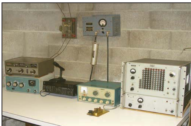
Mike's FMT transmissions will be powered by Heathkit, but the stable source of the signals is Hewlett-Packard instruments, synchronized to GPS satellite time.
